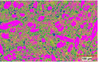
**Remarks:** Microstructure shows the Primary Chromium Carbides and Eutectic Carbides with the Austenite and Martensite.
