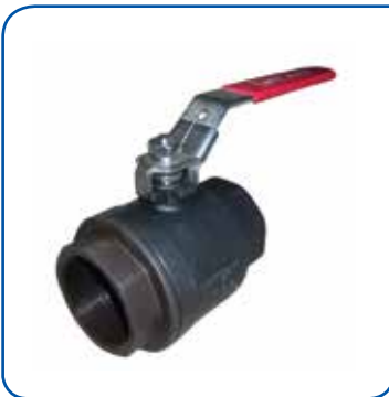
BALL VALVE 2 PC BODY Body : Cast Steel / WCB Size : 1/4" - 4" Conn : BSPT 2000 WOG PTFE Seat
