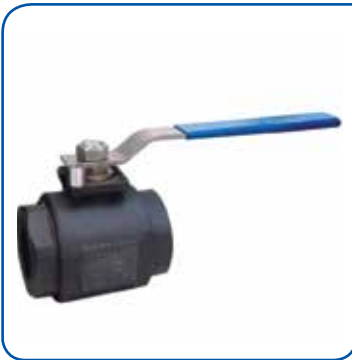
BALL VALVE 2 PC BODY Body : Forged Steel Size : 1/4" - 4" Conn : NPT 2000 WOG With Mounting Pad
