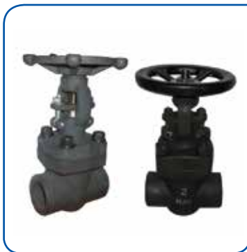
ARITA GATE VALVE Body : Forged Steel/A105/ 304/316/304L/316L Size : 1/2" - 2" Conn : NPT / Socket Weld Class 800 / 1500
