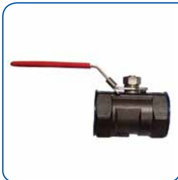
BALL VALVE 1 PC BODY Body : Cast Steel / WCB Size : 1/4" - 4" Conn : BSPT 1000 WOG
