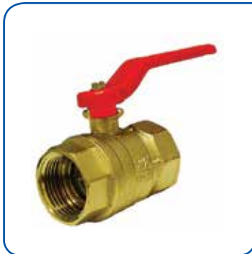
BALL VALVE 1 PC BODY Body : Brass Size : 1/4" - 4" Conn : BSPT 400 WOG Chrome / Without Chrome
