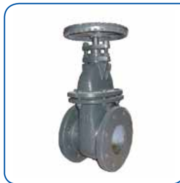
GT GATE VALVE Body : Cast Iron Size : 2" - 12" Conn : JIS 10K Non Rising Stem
