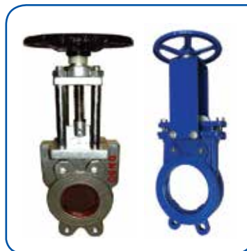
ARITA WAFER TYPE KNIFE GATE VALVE Body : Cast Iron Size : 2" - 24" Conn : JIS 10K, ANSI 150, ANSI 300 Disc : Stainless Steel
