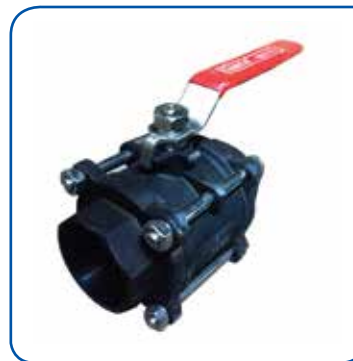
BALL VALVE 3 PC BODY Body : Cast Steel / WCB Size : 1/2" - 4" Conn : BSPT / BW 1000 WOG, PTFE Seat
