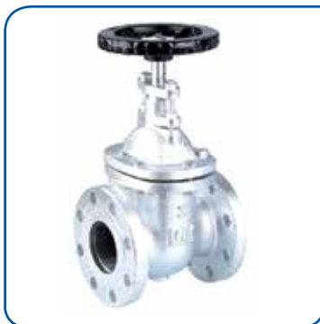
ARITA GATE VALVE 10K Body : Cast Iron Size : 2" - 12" Conn : JIS 10K Non Rising Stem
