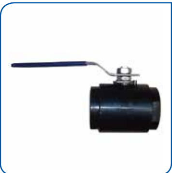
BALL VALVE 1 PC BODY Body : Forged Steel Size : 1/2" - 4" Conn : NPT 6000 WOG PTFE Seat
